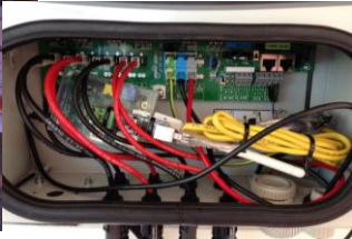
First-generation prototype of ASU Box hooked to solar PV inverter using RS485
