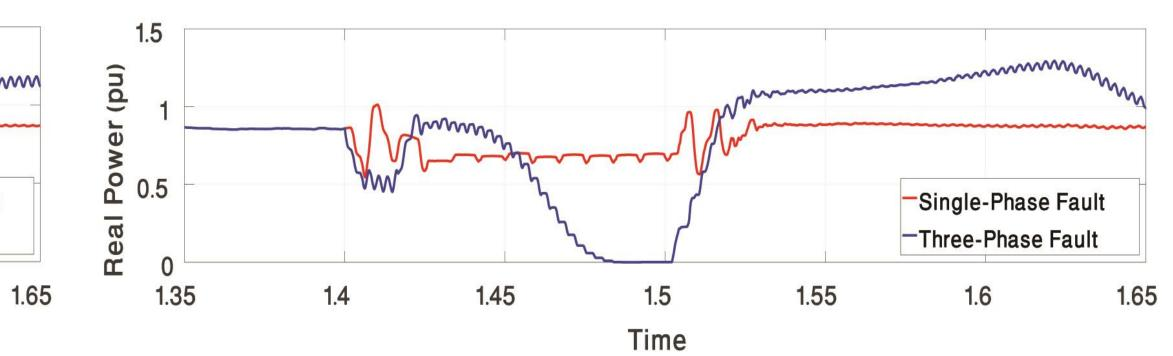
For single-phase the fault, drive a continued to absorb power from the source even at the greatest voltage dip.
