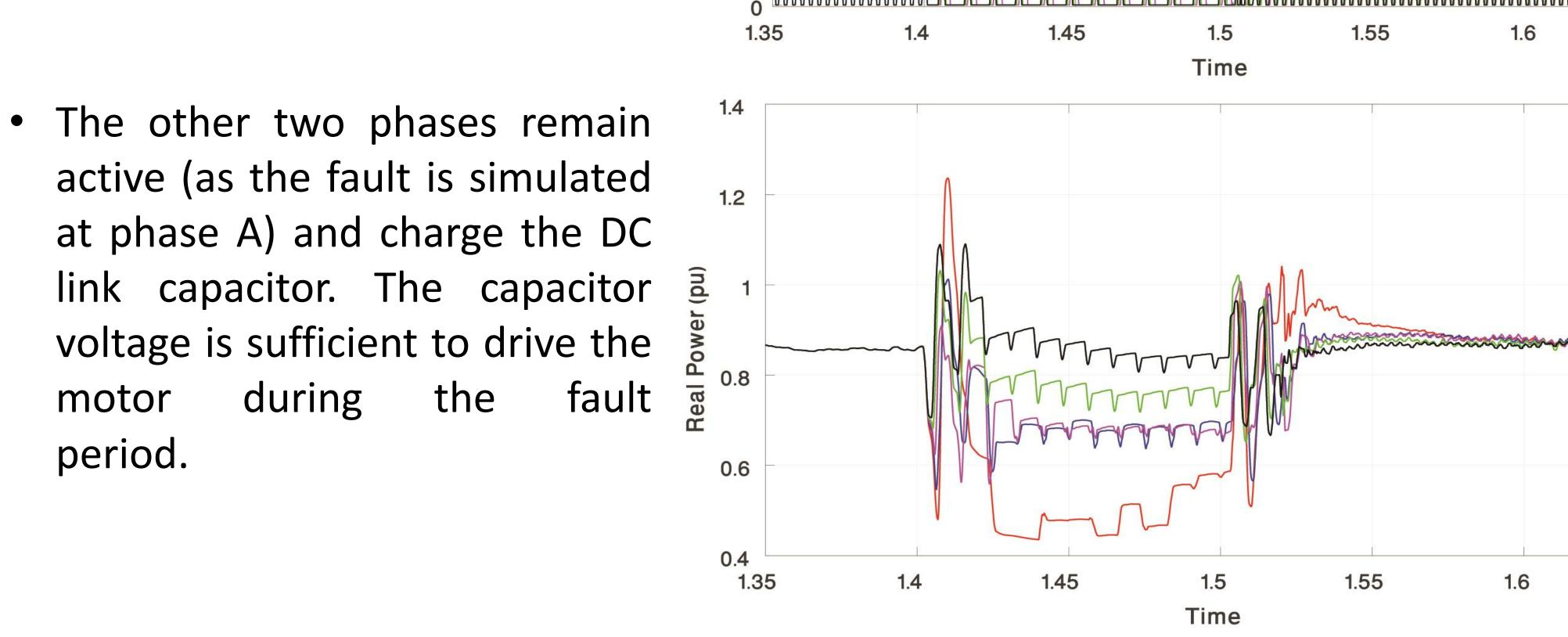
Single-Phase Fault Three-Phase Fault For a three-phase fault, the positive 1.35 sequence power dropped immediately to zero for the case with the greatest voltage dip (53%) and decreased slowly Single-Phase Fault to zero for smaller voltage dips as fault Three-Phase Faul duration increased. 1.35 Time
